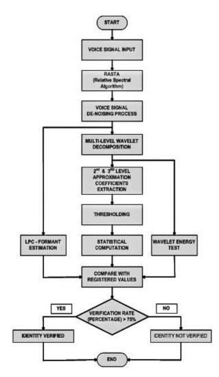
Fig 3.complete System Flowchart.
